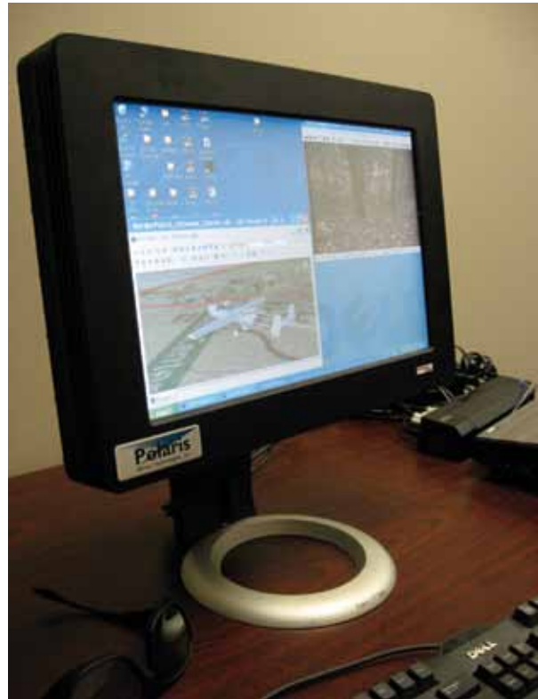
FIGURE 1. Polaris Sensor Technologies' stereo 3-D display uses dual LCD panels in a 1920 \times 1200 -pixel monitor with a 60-Hz refresh rate.
