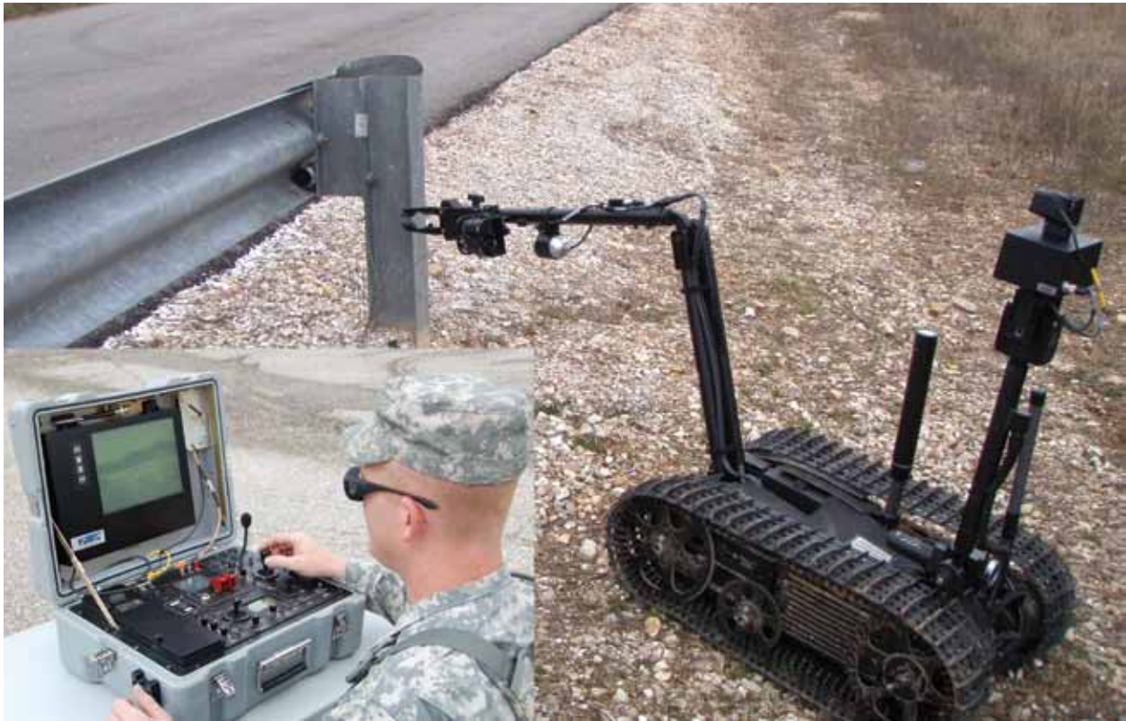
FIGURE 2. Telerobotic systems incorporating stereo cameras are being evaluated by soldiers at Ft. Leonard Wood as a means to provide Explosive Ordnance Disposal technicians a more effective way to deal with improvised explosive devices.
