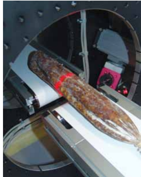
FIGURE 1. To accurately determine the volume of food before it is sliced, a prototype system from ImagingLab uses three structured light sources, three CMOS cameras, and 3-D reconstruction software.
